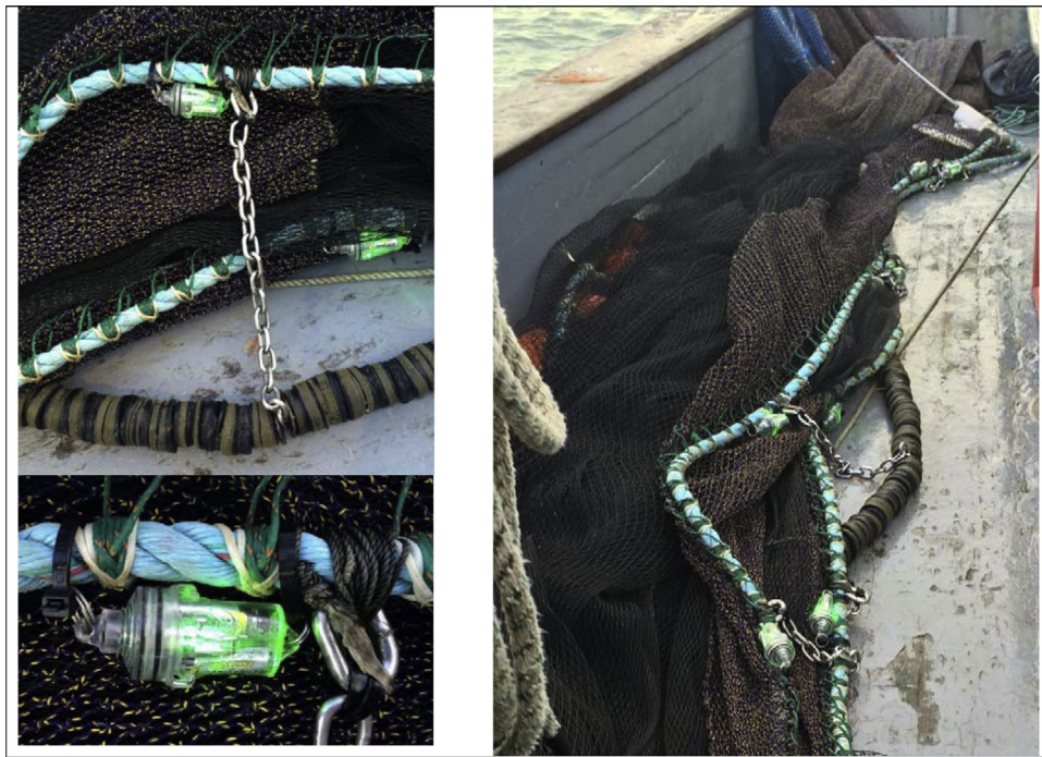
Fig. 2. Image of a green Lindgren-Pitman Electralume® LED light zip-tied to the fishing line of an ocean shrimp trawl (lower left); image of the placement of a green LED in relation to the drop-chains and groundline of an ocean shrimp trawl (upper left); image depicting green LED lights attached to the fishing line of an ocean shrimp trawl prior to trawl deployment (right).
