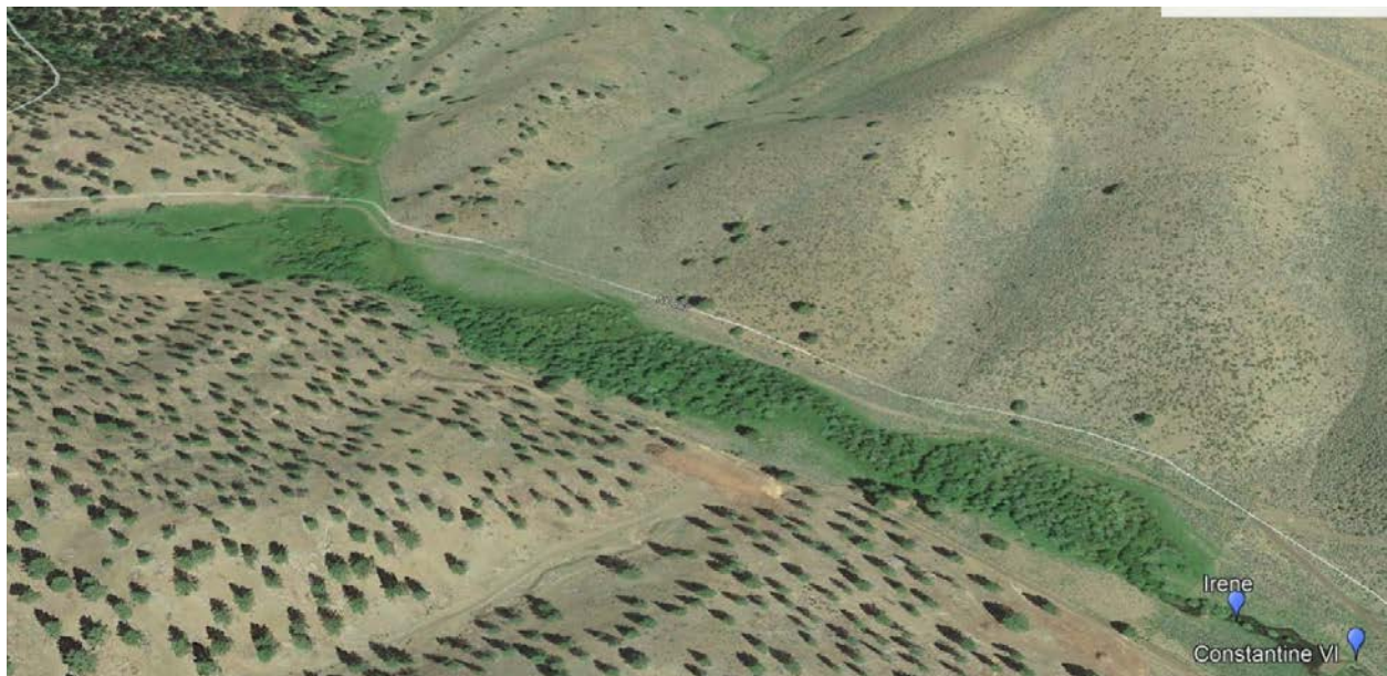
Figure 11. Image of approximately 0.4 mile lengthy of boggy area immediately “upstream” of ABD Irene. There is no channel present in this part of Jump Creek due to small volumes of incoming water, all of which flows subsurface(Google Earth Pro). This boggy area is a natural complete barrier to fish passage, to/from the private and federal lands above the boggy area and to/from the stretch of Jump Creek where ABDs were installed.
