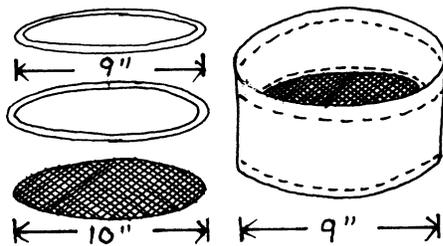
For a collapsible sieve that is easily stored, sew fiberglass screen to a cloth sleeve and attach it to two macrame rings.
