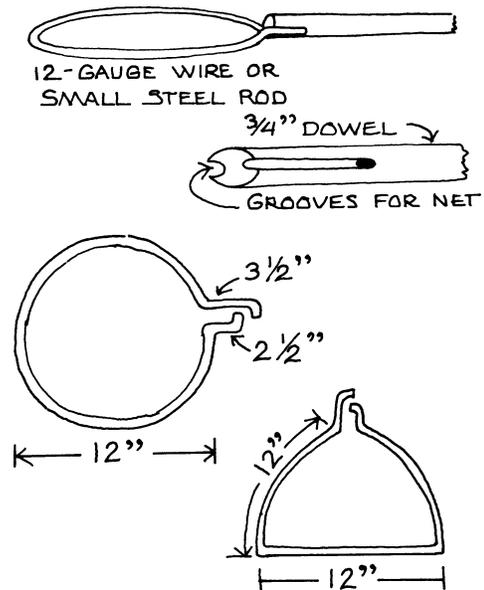
To secure the rim to the handle, wrap the handle with 20-gauge wire, use hose clamps, or find a piece of brass tubing with an interior slightly larger than the dowel to use as a ferrule. Nets can be attached by sewing them onto the rim, sliding them onto the rim (you need ferrules for this), or attaching with grommets and hog rings.
