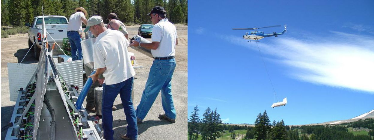
Air stocking trout in high mountain lakes. Left – loading fish into the air stocking tank. Right – the air stocking tank airborne near Mt. Hood.
