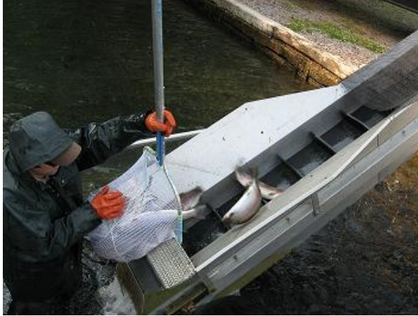
Using a fish lift at Klamath Hatchery to load rainbow trout for stocking
