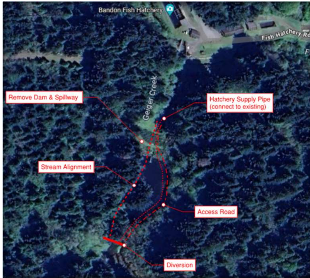
Figure 3.1 – Bandon – Proposed Geiger Creek Dam Relocation
