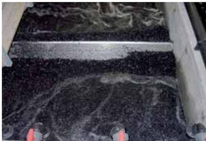
Figure 10. Fluid bed filter
