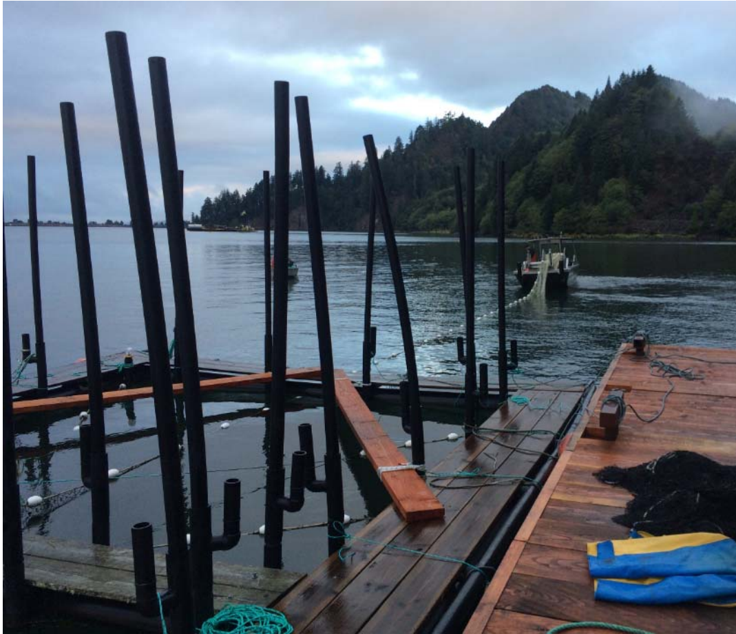
Figure 9g. Hearts and lead of experimental floating fish trap (looking downstream) near Jim Crow Creek, Washington, 2016.
