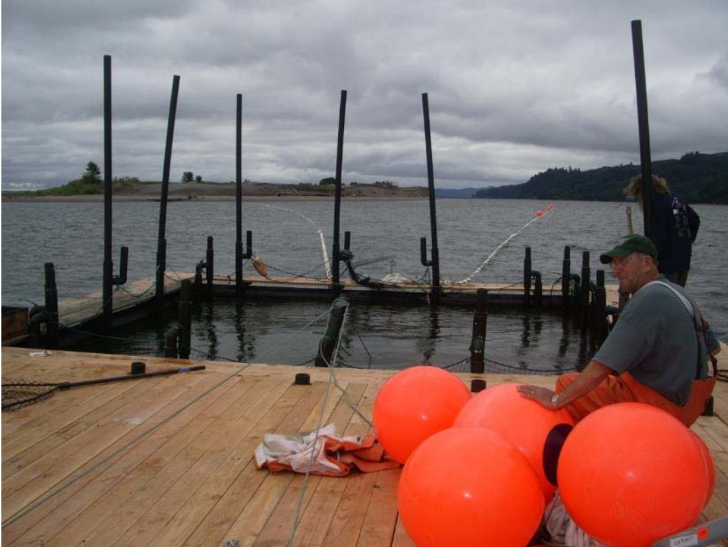
Figure 9d. Leads (in background) and pot on experimental floating fish trap, 2010.
