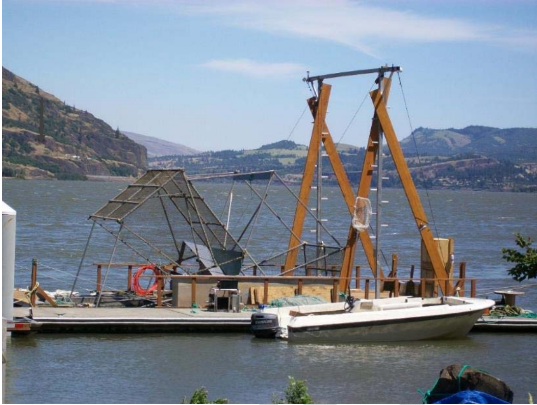
Figure 13c. A modern-day experimental fish wheel, much smaller in size than its predecessors, located in the Columbia River Gorge.
