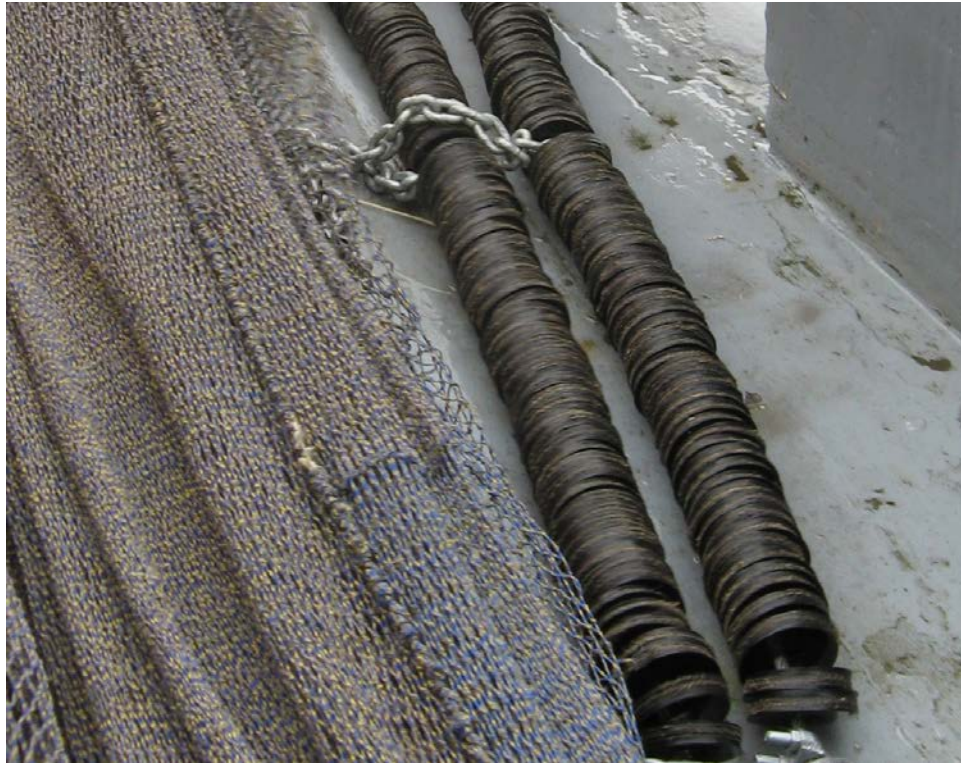
Figure 3. Picture showing the disk-covered central groundline sections used in experiment 2.
