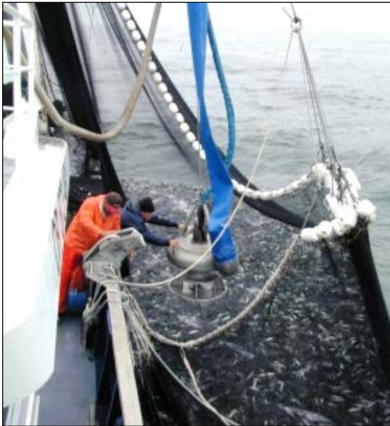
Fishers prepare to suck sardines from a seine net into the hold.
