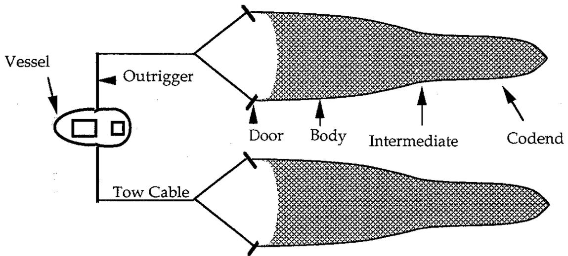
Figure 1. Schematic of a double-rigged shrimp vessel with net body, intermediate and codend sections indicated.
