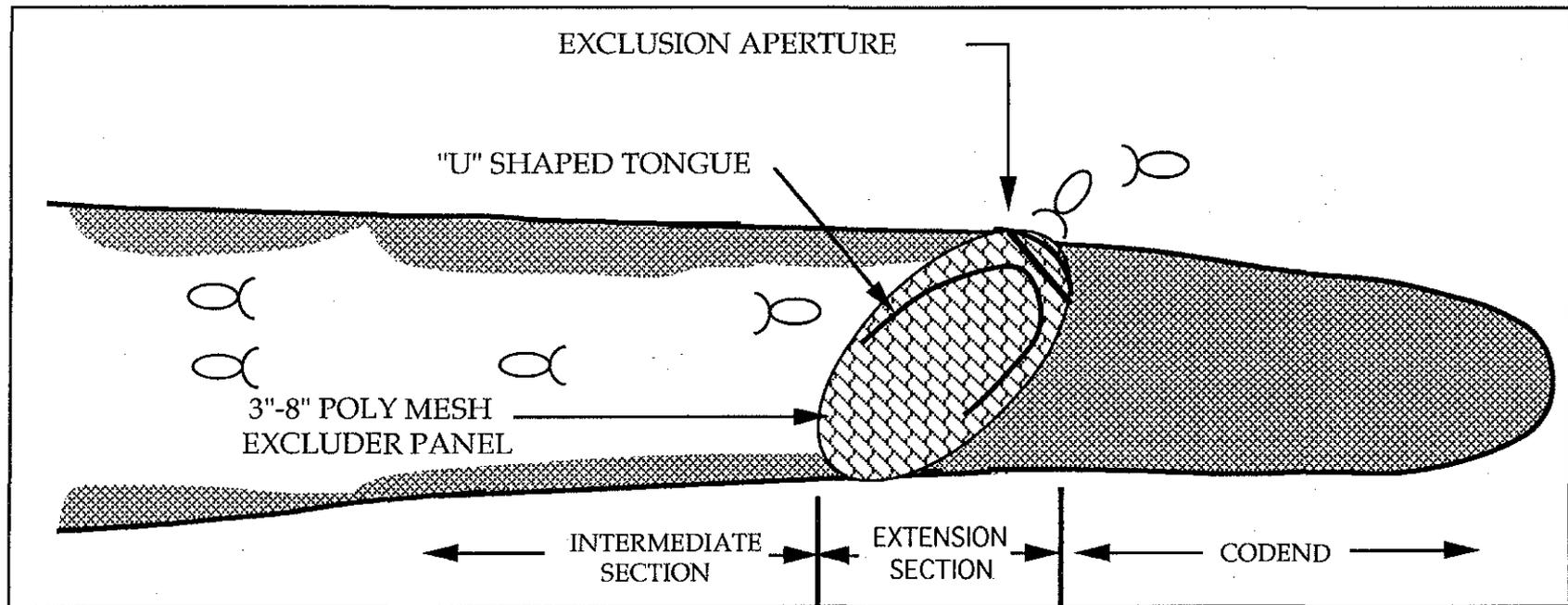
Figure 2. Diagram of an enabled soft mesh panel fish excluder installed in a ocean shrimp trawl. The device is mounted in an extension section, placed between the intermediate of the trawl and the codend. The device is disabled by unlacing the "U" shaped tongue and lacing the exclusion aperture closed.
