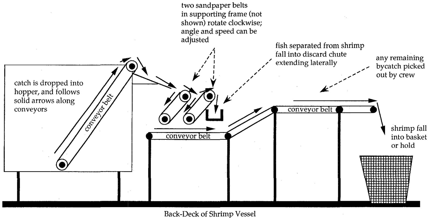
Figure 7. Diagram of back-deck shrimp handling equipment, including the "smelt belt" (rotating belts and discard chute). As the catch falls onto the first belt, smaller fish tend to stick to the belt while shrimp slide down onto the conveyor below. The process is repeated on the second belt, with anything sticking to the belt entering the discard chute. Small shrimp and molting shrimp tend to stick to the sandpaper belts more readily than larger shrimp, sometimes ending up in the discard chute.
