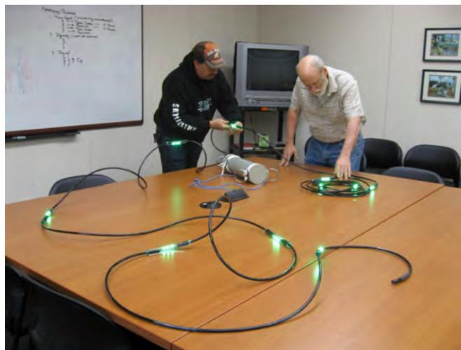
**Figure 21. ODFW shrimp project leader Bob Hannah (right), views an early version of the LED light system developed by Cory Rock (left), owner and skipper of the F.V. Kylie Lynn. He's worked out a number of "bugs" that led to design changes, but says the current system is working well and is holding up to the rigors of trawling.**
